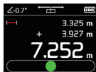
When taking a new measurement, the instrument automatically adds the data and sums them up
